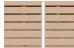
In the case of end-to-end joints, we recommend covering the joint. This can be achieved with customary aluminium T-rails. Otherwise, varying changes in length could lead to a slightly irregular joint pattern.
