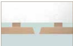
concealing the hollow chamber by means of bevel cut
