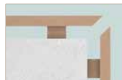
open miter joint
