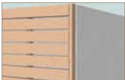
covering the hollow chamber with end plate
