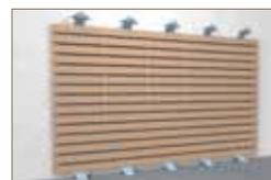
Due to Resysta's high diffusion resistance, a rear ventilation of the facade is always required. The rear ventilation distance must measure at least 20 mm and may not be reduced. The air inlet opening and venting opening must be 20 mm wide end-to-end.
