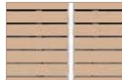
In the case of end-to-end joints, we recommend covering the joint. This can be achieved with customary aluminium T-rails. Otherwise, varying changes in length could lead to a slightly irregular joint pattern.
