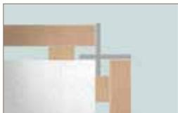
open corner with standard aluminium end plate
