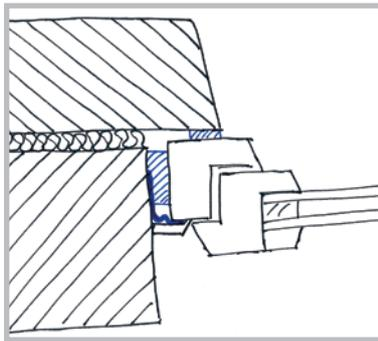
Checked rebate at the side (double-wall masonry)
