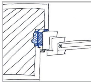
Checked rebate at the side (monolithic masonry)
