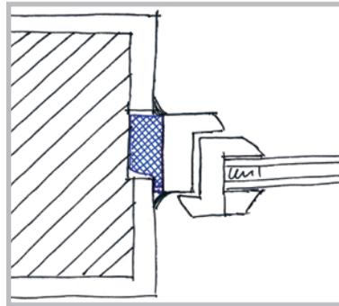
Uneven rebate at the side (monolithic masonry)
