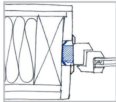
Uneven rebate at the side (timber-frame construction)
