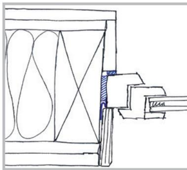
Uneven rebate at the side (timber-frame construction)
