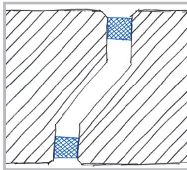
Solid wall construction joint (schematic layout)
