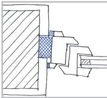
Uneven rebate at the side (monolithic masonry)
