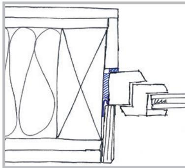
Uneven rebate at the side (timber-frame construction)
