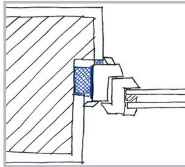
Checked rebate at the side (monolithic masonry)
