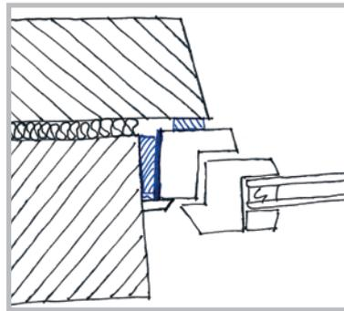
Checked rebate at the side (double-wall masonry)
