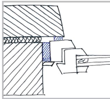
Checked rebate at the side (double-wall masonry)
