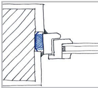
Uneven rebate at the side (monolithic masonry)
