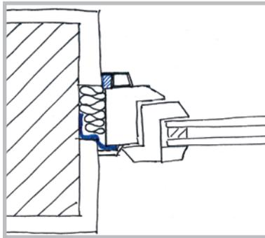
Uneven rebate at the side (monolithic masonry)
