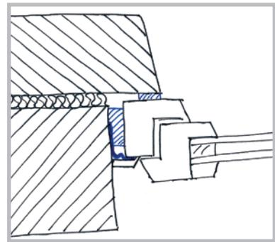
Checked rebate at the side (double-wall masonry)
