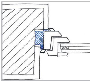
Checked rebate at the side (monolithic masonry)
