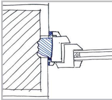
Uneven rebate at the side (monolithic masonry)
