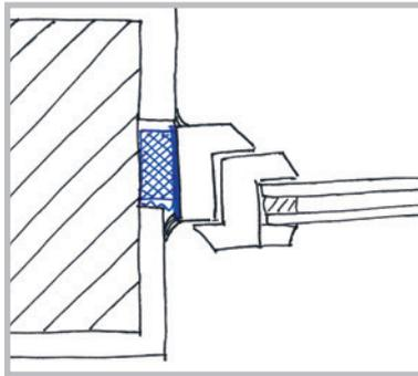
Uneven rebate at the side (monolithic masonry)
