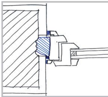
Uneven rebate at the side (monolithic masonry)
