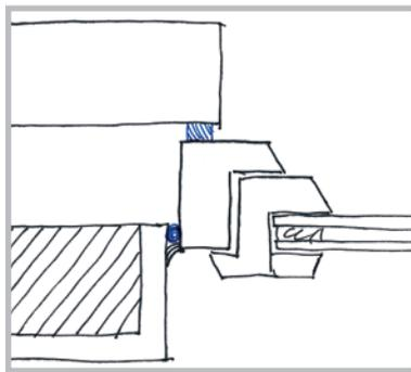
Checked rebate, faced with brickwork / block work
