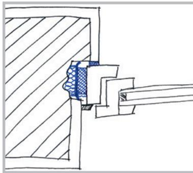
Checked rebate at the side (monolithic masonry)
