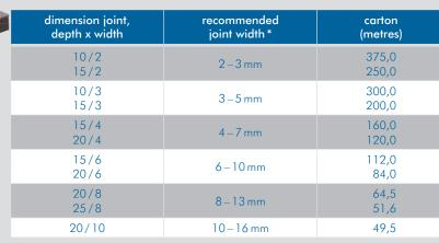
\* Movement in structural elements and temporary longitude changes are to be taken into account by the max. joint width.
